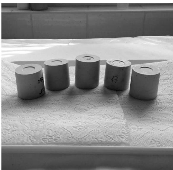
Fig. 13 SIAL<sup>®</sup> samples of sodium sulfate simulated liquid waste (1.5 years later)
