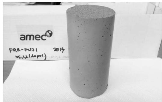
Fig. 10 SIAL<sup>®</sup> sample of ion-exchange resin after thermal treatment (2 years later)
